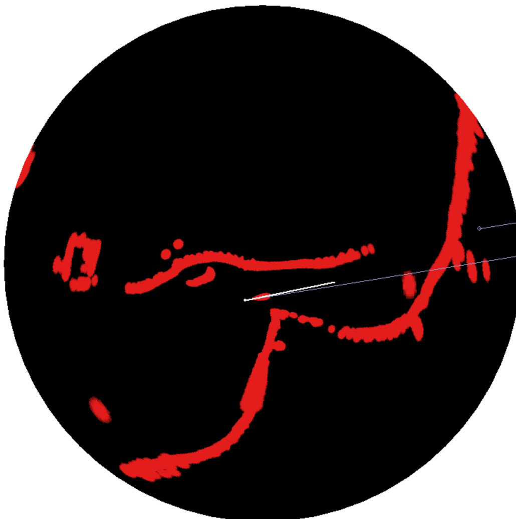
Figure 6.50. Display on the radar PPI of the entire navigation situation around the vessel, observed when approaching the Verkhny Pellovsky range line
