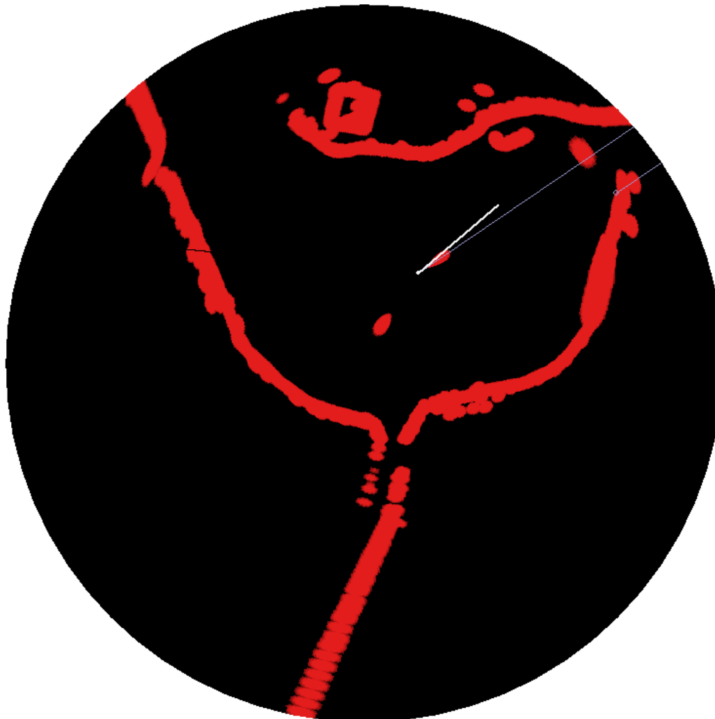
Figure 6.47. Display on the radar PPI of the entire navigation situation around the vessel, observed when approaching the Verkhneporozhsky range line
