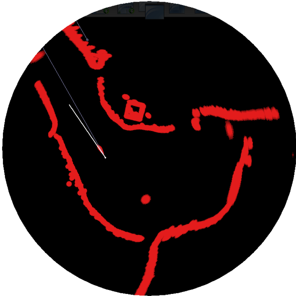
Figure 6.40. Display on the radar PPI of the entire navigation situation around the vessel, observed when moving along the Tosnensky range line
