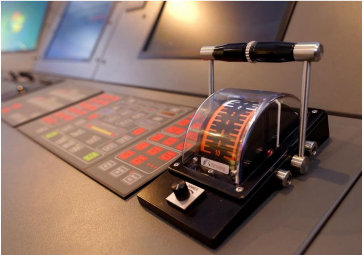
Figure 6.2. Engine telegraph and control panels of the vessel of the Transas NTPro 4000 navigation simulator
