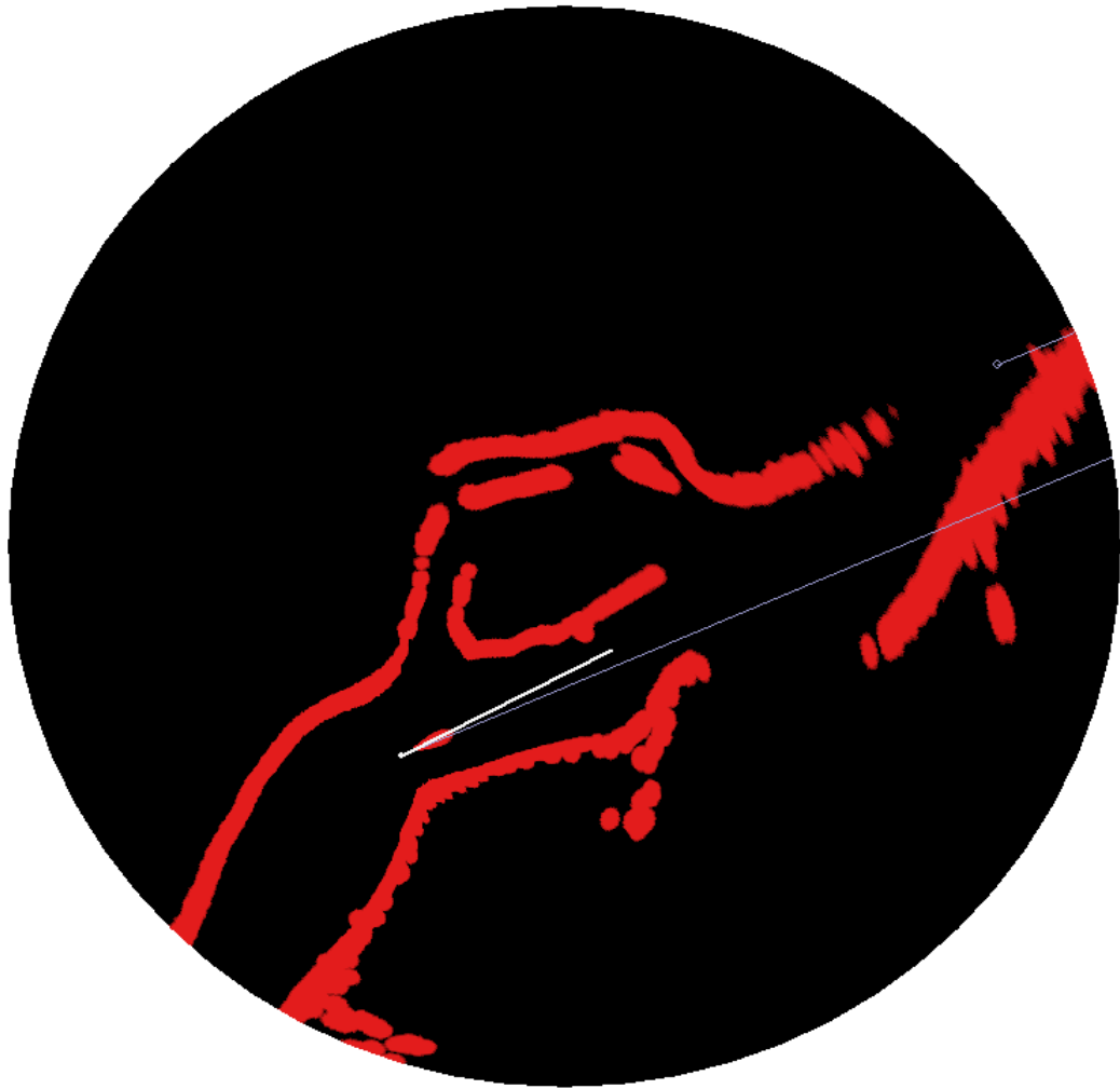
Figure 6.55. Display on the radar PPI of the entire navigation situation around the vessel, observed during curvilinear movement when approaching the Nizhny Pellovsky range line
