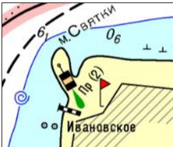
Figure 3.6 Visual sign on the left bank
