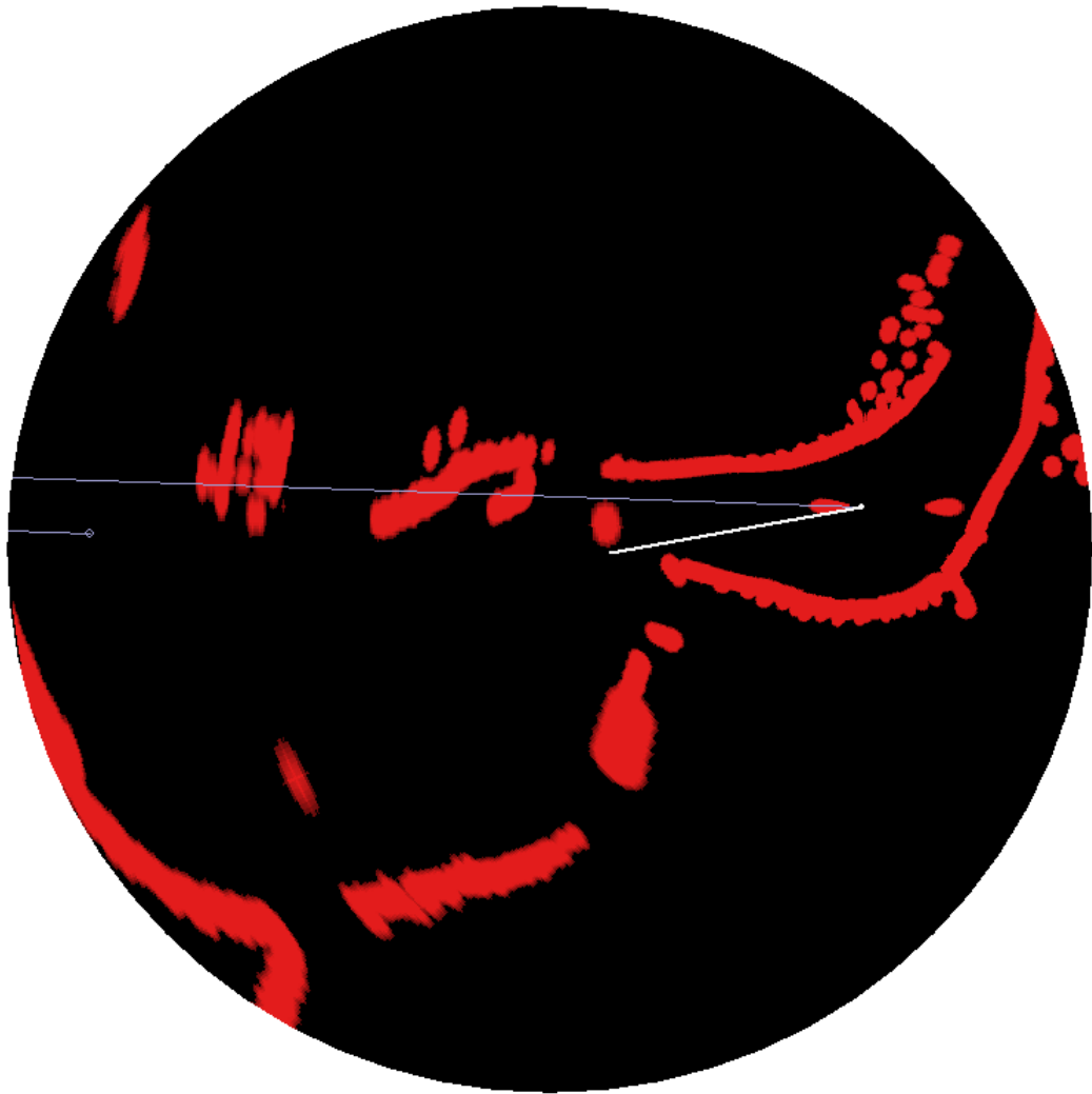
Figure 6.39. Display on the radar PPI of the entire navigation situation around the vessel, observed at the time of the change in the direction of the vessel speed vector when moving along the Verkhny Pellovsky range line
